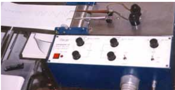
FIGURE 5 - Device used to perform the active anterior rhinomanometry exam. Rhinomanometer RM - 302 from Berger™.
